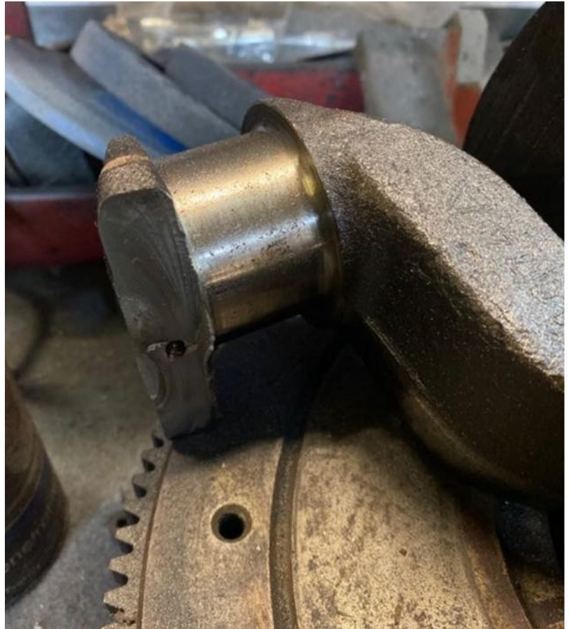
The MGA's broken crankshaft
