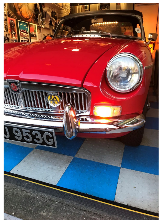
Front indicator and side lights fitted.
