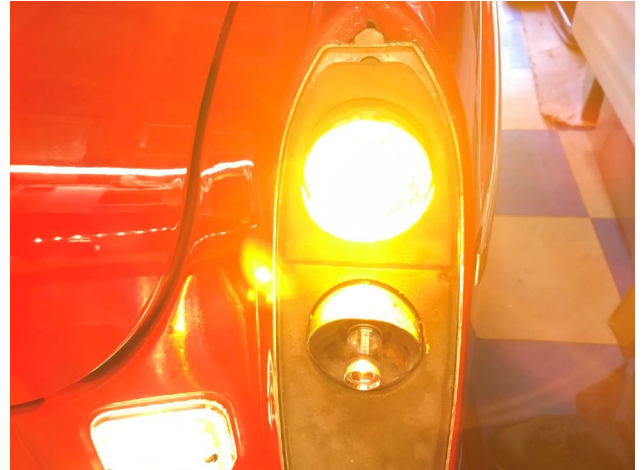
Rear indicator/stop/tail LED bulbs fitted. A bit brighter than standard, but fitting the lens unit calms it down.
