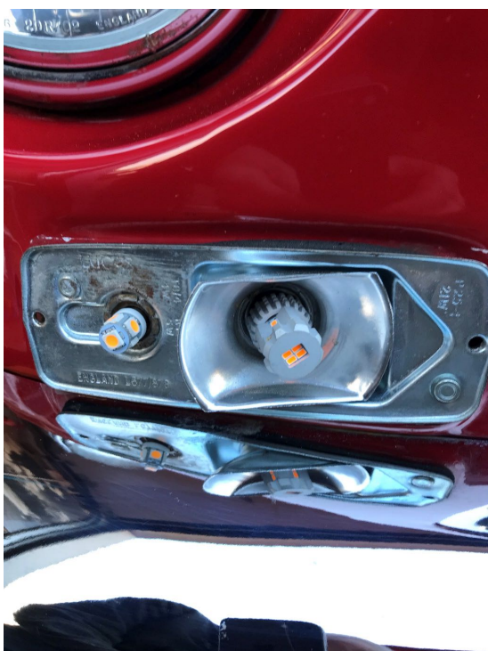
Front indicator and side lights fitted.
