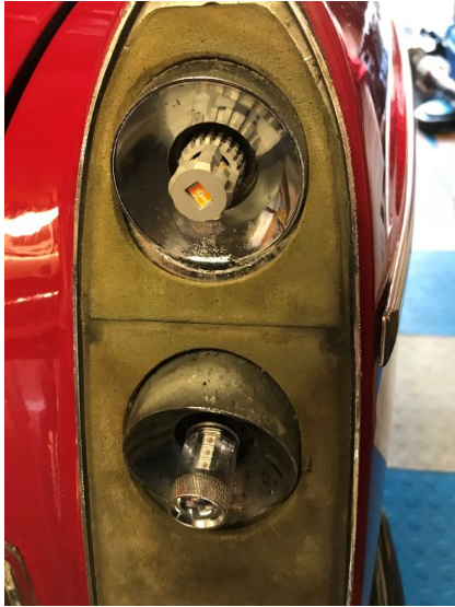
Rear indicator/stop/tail LED bulbs fitted. A bit brighter than standard, but fitting the lens unit calms it down.
