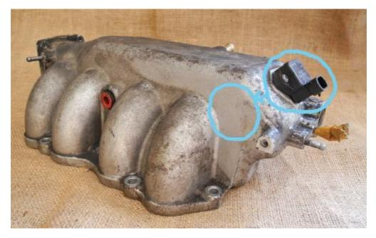
First thing to do was to check I could remove the sensor, normally I'm used to UNF nuts and bolts, but this being a modern car you would expect metric nuts but no - they are now using torx heads. This coupled with steel screws into an alloy manifold did not bode well. However, after a liberal dose of WD40, they came undone and revealed a "a long pokey bit with a seal on it" of approx. 25mm.
